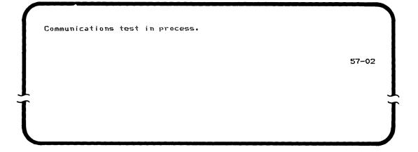
This display may stay on the screen for as long as 30 seconds. If the display does not change after that time, an error has occurred from which the system cannot recover. Call your service representative.
