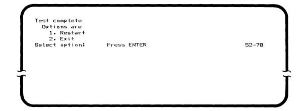
7. You may test other keyboards and any magnetic stripe readers by selecting option 2 which takes you back to the prompt for program name. At the next keyboard, repeat "Part 1 (Keyboard)" on page 14. Continue repeating this part until you have completed testing all keyboards.
