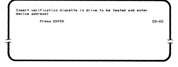
9. Move the verification diskette to the drive to be tested if necessary, and enter the device address of the diskette drive to be tested. Press the ENTER key.
